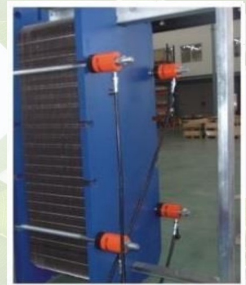
4 EAGLE PRO ESH-306 pulling threaded bar in a large heat exchanger
