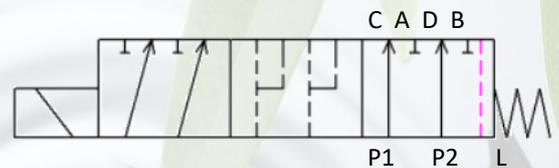
Operation and hydraulic schemes Selector valves type DVS6 with direct solenoid operation, control the direction of the hydraulic medium flow. They are mostly used as link between two consumers and the basic directional valve, when we want to control both consumers alternately by means of one basic directional valve.
