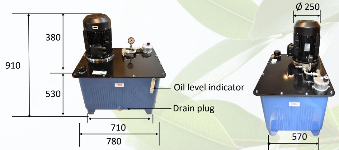
This Hydraulic Power Unit comes with a double pump at 11+14 cm<sup>3</sup> with high/low function.
